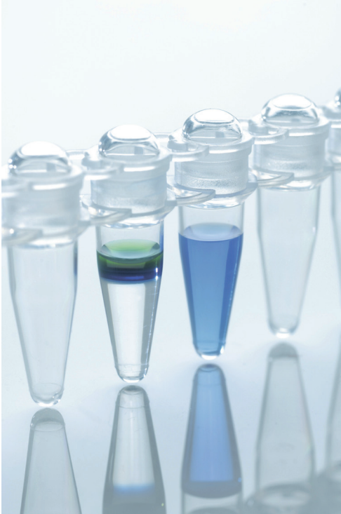
Figure 1. The DNA Protect Buffer for the EpiTect Fast Bisulfite kits. The buffer contains a pH indicator dye as a mixing control. It also enables confirmation of the correct pH for cytosine conversion.
